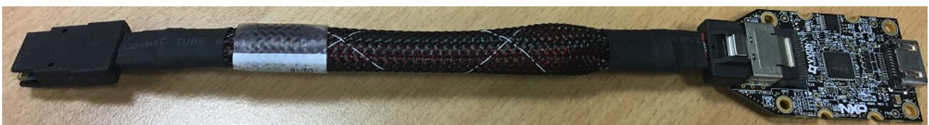
Figure 3. i.MX mini SAS cable with LVDS-to-HDMI adapter
