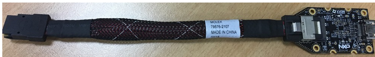
Figure 2. i.MX mini SAS cable with DSI-to-HDMI adapter
