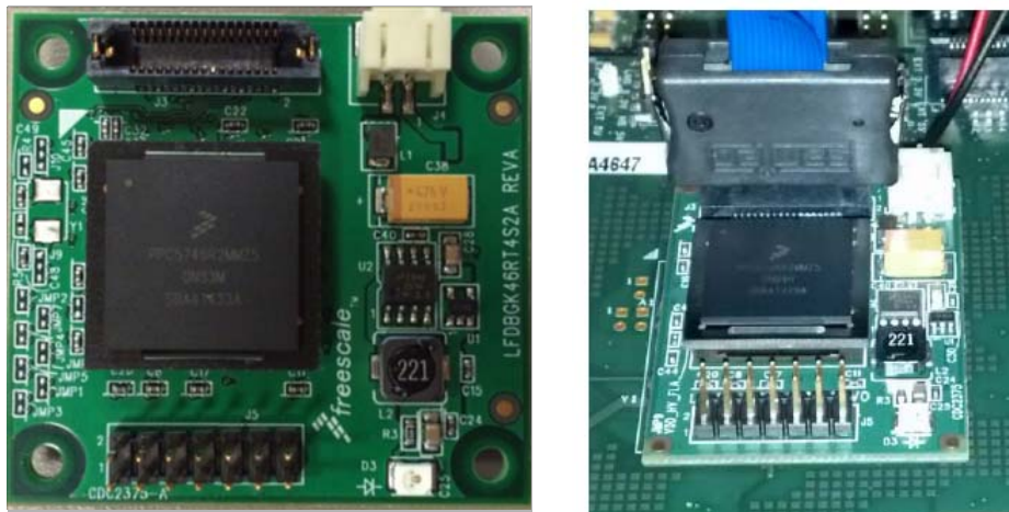
Figure 19. 292 BGA to 252 PGA Adapter card for Emulation and Debug Device
