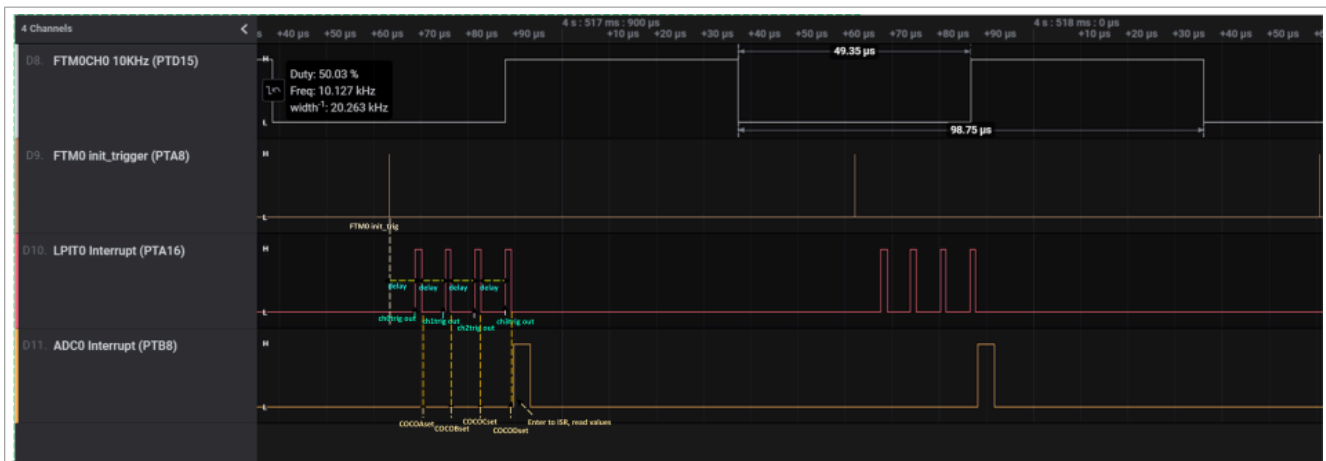
Figure 8. Timing of LPIT0 trigger for four ADC channels in this use case
