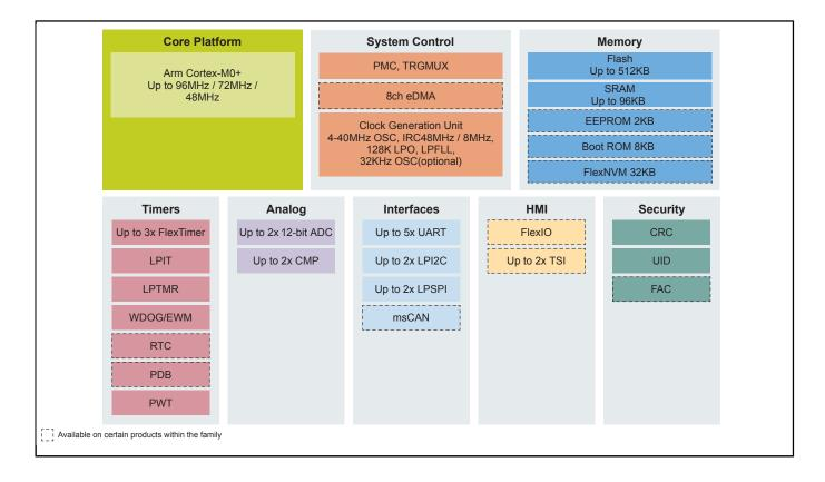
View additional information for KE1xZ: Arm® Cortex®-M0+ 5V Main Stream MCU with NXP Touch and CAN Control.
