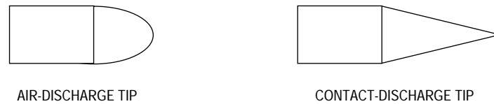
Figure 10. Example of Air-Discharge and Contact-Discharge Tips
