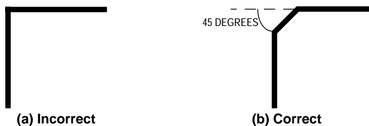
Figure 7. Incorrect (a) and Correct (b) PCB Track Layout for HCMOS Designs
