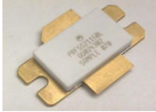
Figure 2. PRF5S21150L 150 W Device in a Cu Laminate Low Rth Package
