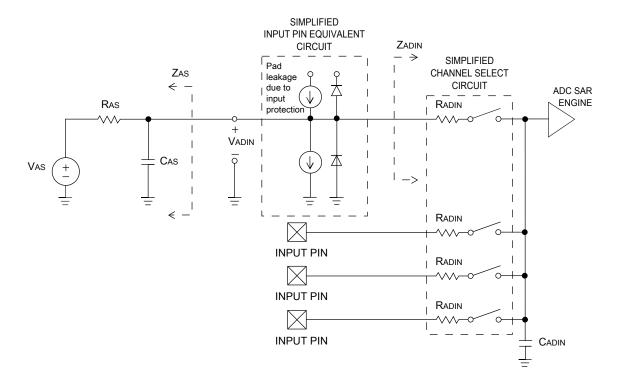
Figure 19. ADC input impedance equivalency diagram
