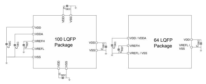
Figure 13. Pinout decoupling
