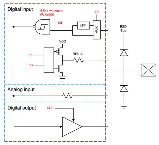
Figure 5. I/O simplified block diagram
