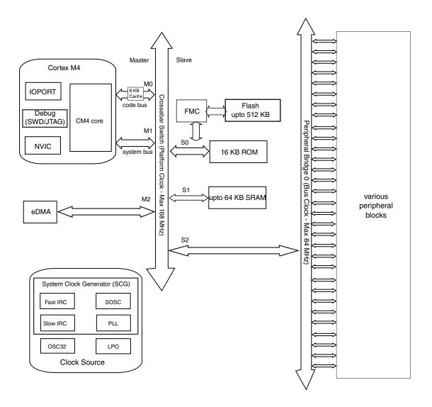
Figure 2. System diagram
