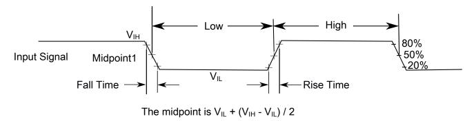
Figure 16. Input signal measurement reference
