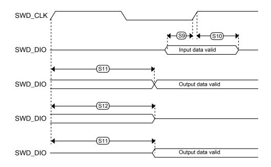
Figure 29. Serial wire data timing
