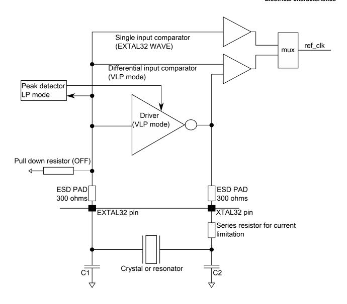
Figure 17. Oscillator connections scheme (OSC32)
