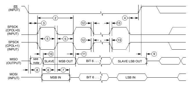
Figure 27. LPSPI slave mode timing (CPHA = 1)
