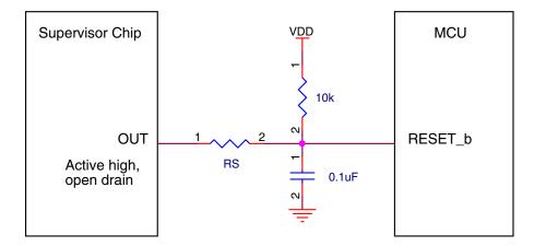
Figure 37. Reset signal connection to external reset chip
