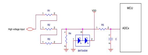
Figure 35. High voltage measurement with an ADC input
