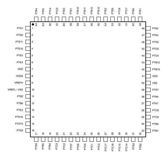
Figure 8. 64 LQFP Pinout Diagram
