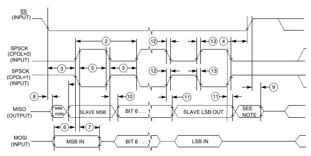
Figure 26. LPSPI slave mode timing (CPHA = 0)
