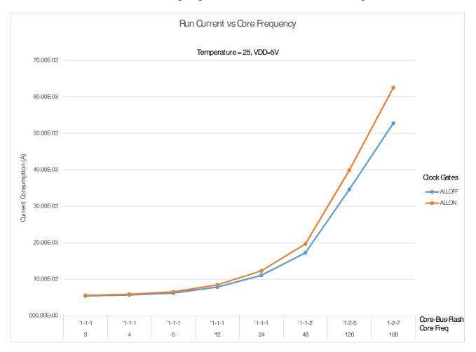
Figure 14. Run mode supply current vs. core frequency
