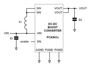
**Figure 4.** DC-DC Converter requires only three external components.
