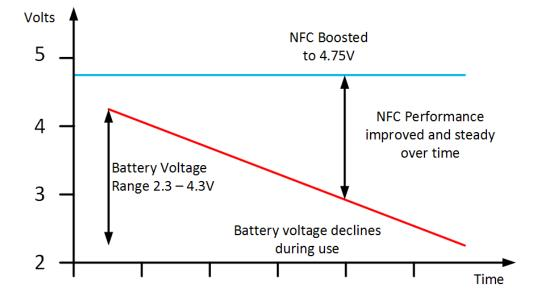
Figure 2. DC-DC Boost delivers steady and strong NFC field.
