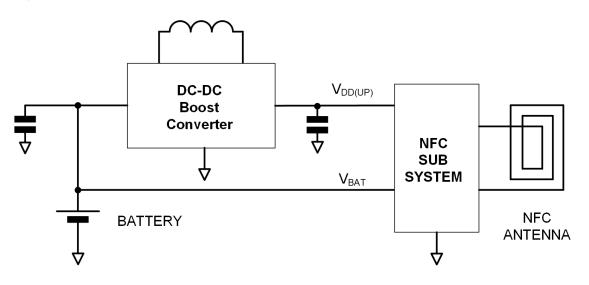
Electrical noise is the enemy of many radio systems found in a smartphone. By reducing noise in the relevant bands from 10 KHz to 1.5 MHz, these DC-to-DC Boost Converters improve the performance of those other radio receivers within the mobile device.
