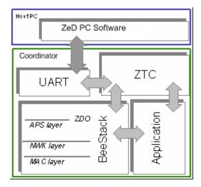
Figure 1-2. Interface Between ZeD Coordinator and ZeD PC Software
