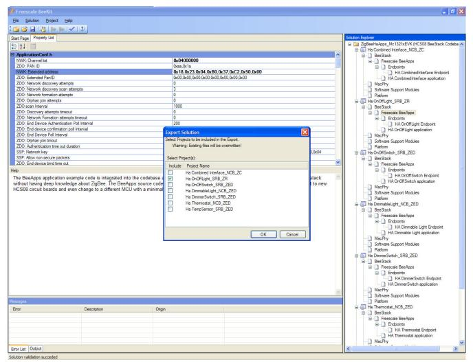
Figure 2-2. ZeD ZigBeeHaApps\_MC1321xEVK BeeKit Solution
