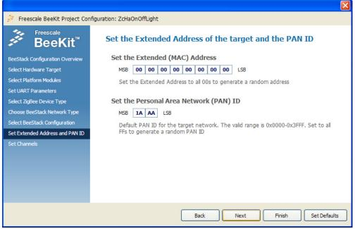
Figure 3-11. Extended Address and PAN ID Selection Page
