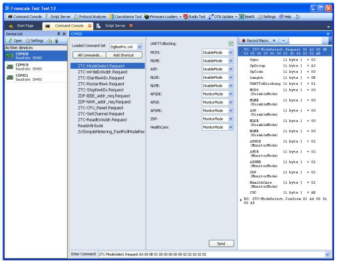
Figure 6-3. ZTC-ModeSelect.Request Command (Confirm Communication)
