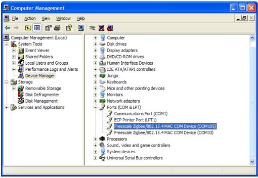
Figure 5-20. COM Ports in Device Manager
