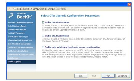
Figure 10-1. Enabling OTA Cluster Server on SE Energy Service Portal Coordinator
