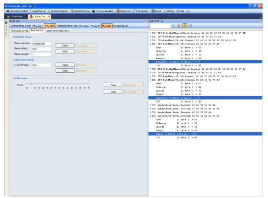
Figure 7-5. Device Memory Commands and PA Level Set
