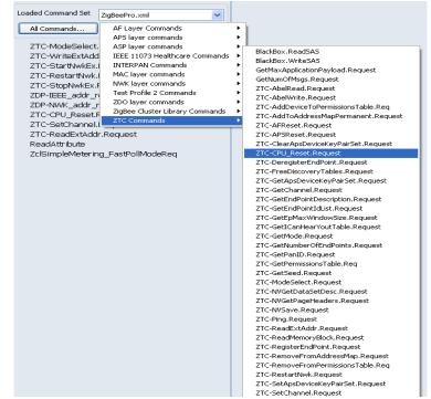
Figure 2-29. Selecting a Command from the Command Set
