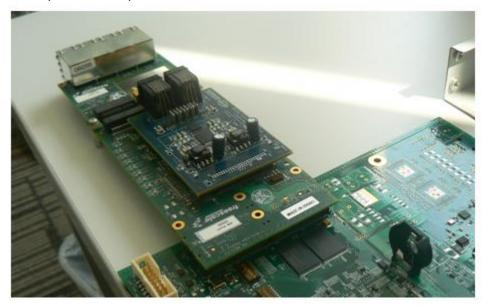
Figure 11 Insert T1/E1 PMC card and Voice card
