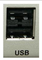
Figure 4: Dual USB Ports on P1025RDB-PA
