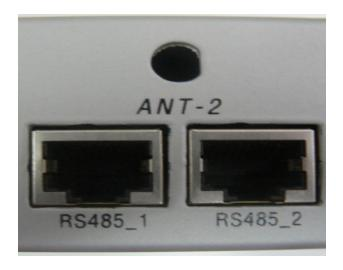
Figure 6: RS485 ports on P1025RDB-PA
