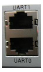
Figure 5: UART Ports on P1025RDB-PA
