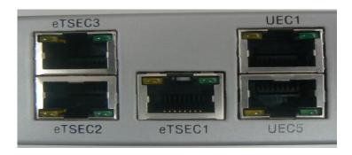
Figure 3: Ethernet Ports on P1025RDB-PA
