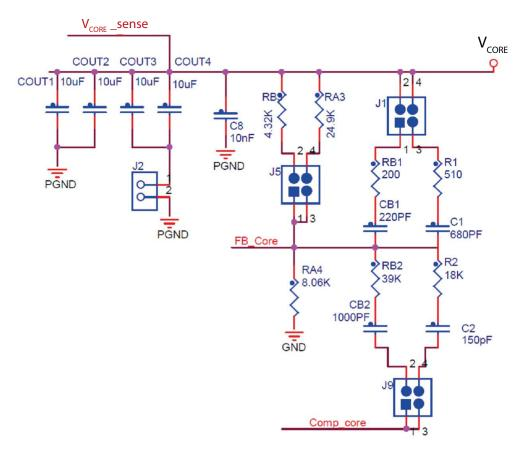
Figure 4. Compensation Network and V<sub>CORE</sub> Setup Schematic
