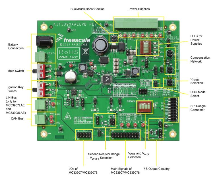
Figure 2. Block Diagram for KIT33907LAEEVB and KIT33908LAEEVB
