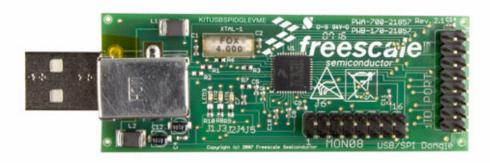
Figure 6. KITUSBSPIDGLEVME Interface Dongle
