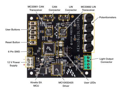
Figure 1: Front side of KEA128LEDLIGHRD
