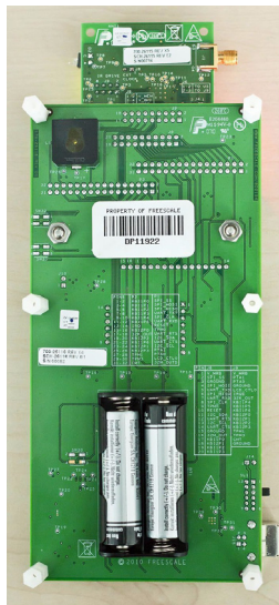
Figure 5. 1323x-RCM Board Back with Batteries Installed
