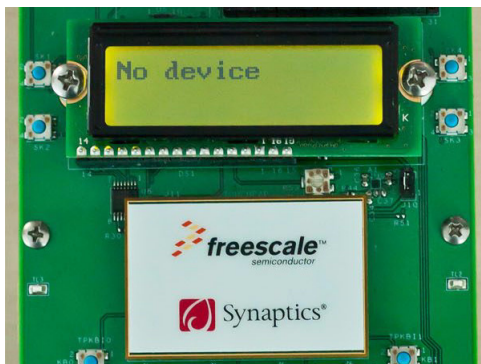
Figure 6. 1323x-RCM Initialized Board
