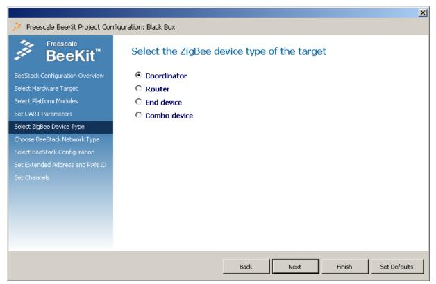
Figure 7-3. Device type selection window.
