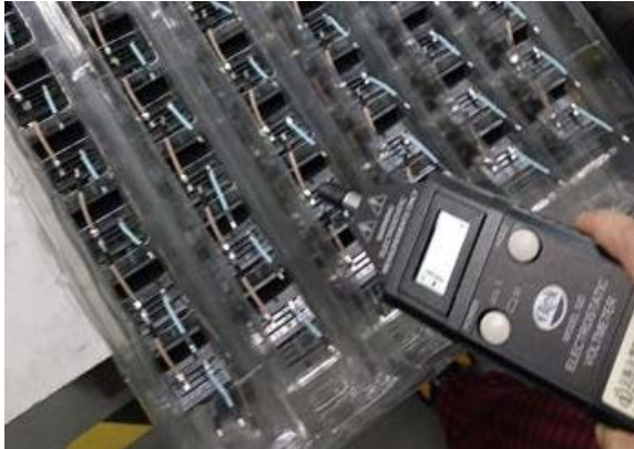
Example non ESD safe components.
