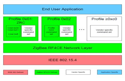
Figure 1-1. Application Software Protocol Stack
