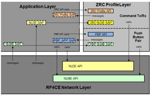
Figure 2-1. Freescale ZRC Profile layer components and Interfaces
