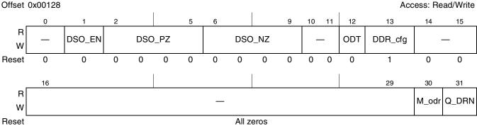
Figure 5-15. DDR Control Driver Register (DDRCDR)
