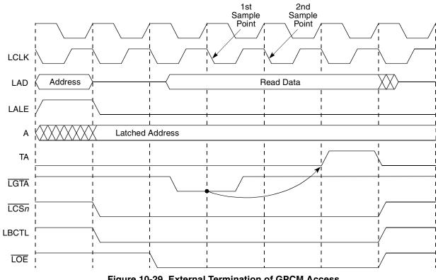
Figure 10-29. External Termination of GPCM Access
