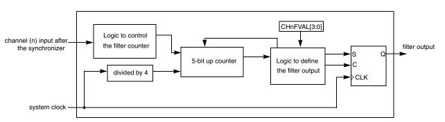
Figure 11-33. Channel Input Filter
