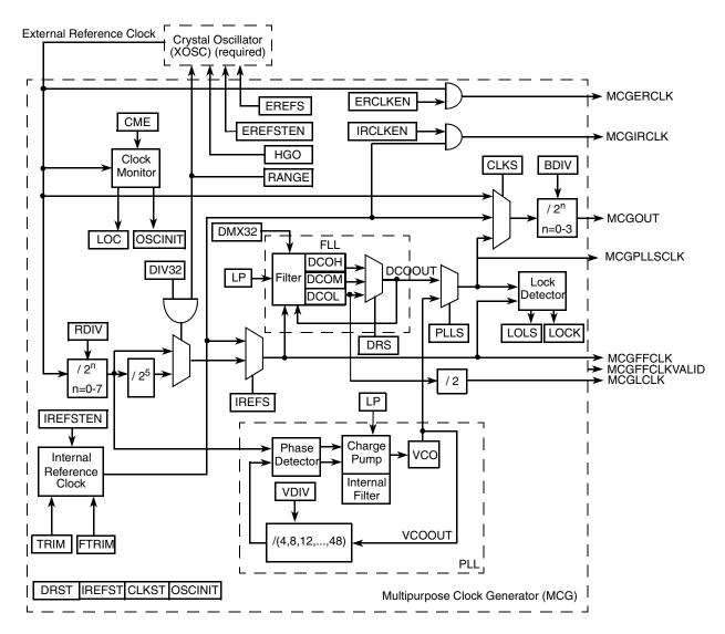
Figure 16-1. Multipurpose Clock Generator (MCG) Block Diagram
