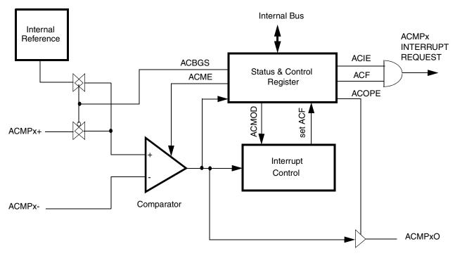
Figure 8-1. Analog Comparator 5 V Block Diagram
