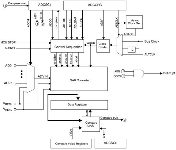
Figure 9-1. ADC Block Diagram
