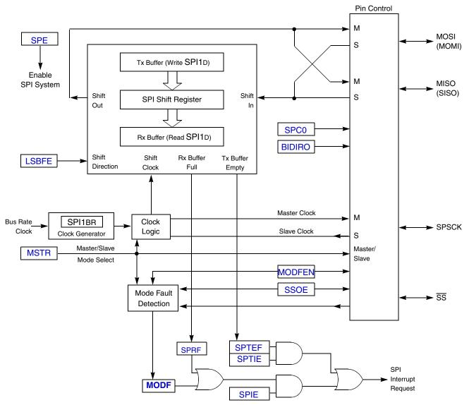
Figure 19-2. SPI Module Block Diagram
