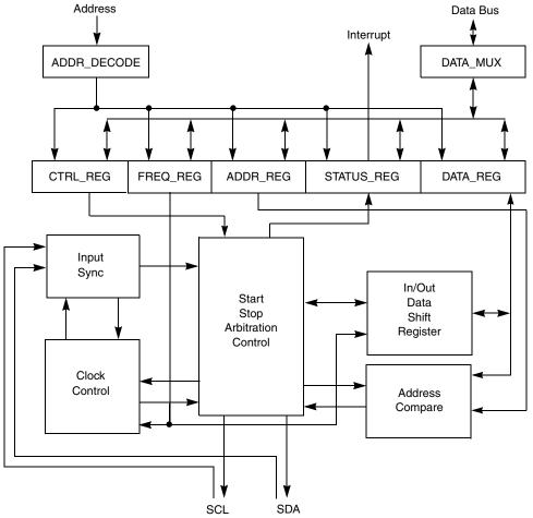
Figure 12-1. IIC Functional Block Diagram
