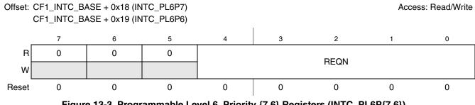
Figure 13-3. Programmable Level 6, Priority {7,6} Registers (INTC\_PL6P{7,6})
