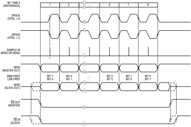
Figure 20-17. SPI Clock Formats (CPHA = 0)
