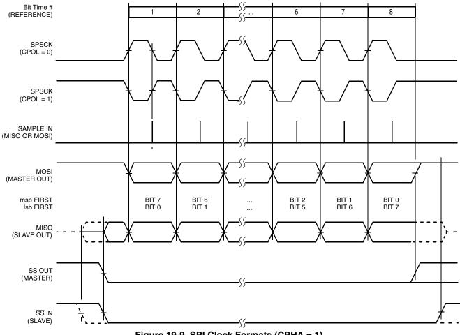
Figure 19-9. SPI Clock Formats (CPHA = 1)
