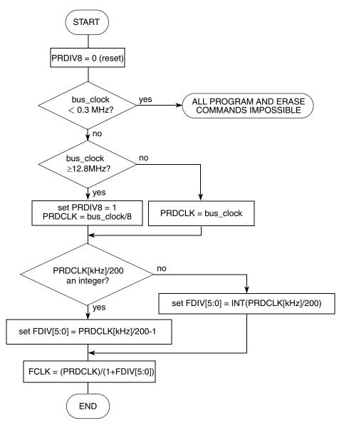
Figure 4-9. Determination Procedure for PRDIV8 and FDIV Bits
