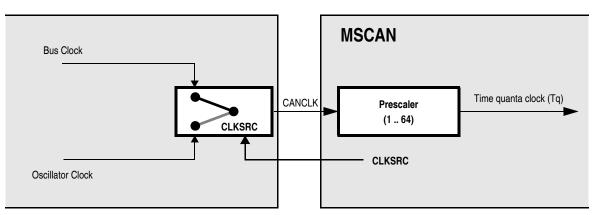
Figure 15-41. MSCAN Clocking Scheme
