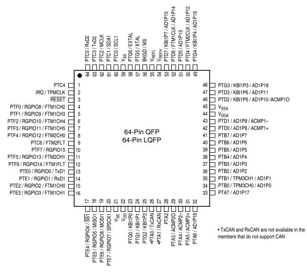
Figure 2-2. 64-Pin LQFP/QFP
