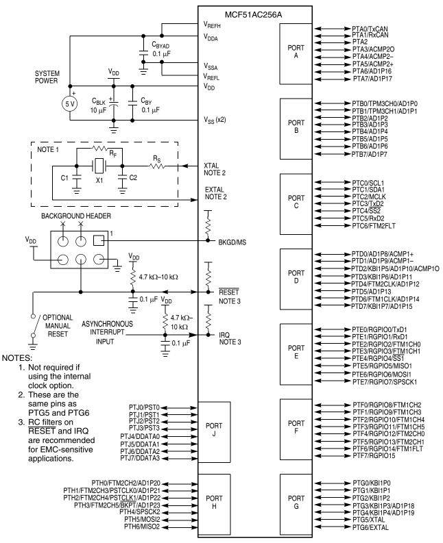
Figure 2-4. Basic System Connections
