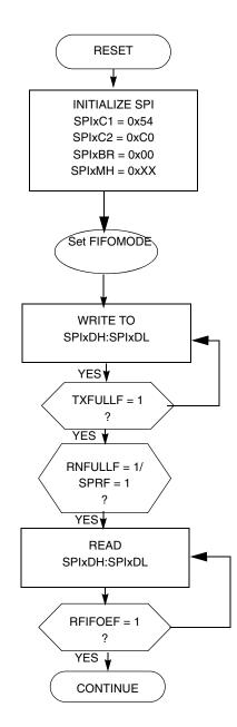
Figure 20-20. Initialization Flowchart Example for SPI Master Device in 16-Bit Mode for FIFOMODE
