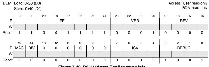
Figure 7-12. D0 Hardware Configuration Info
