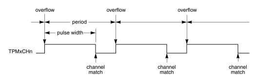
Figure 21-14. EPWM period and pulse width (ELSnA=0)
