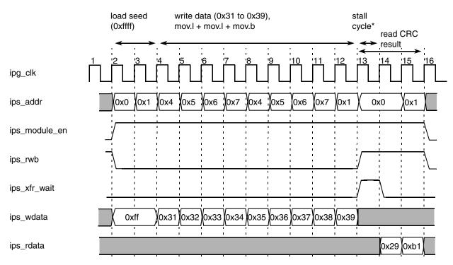
\* On cycle 13, there is a read-after-write hazard, since calculation of 0x39 data is underway. *ips\_xfr\_wait* is asserted to signalize a stall cycle (the IPS master must wait until cycle 14 to read the CRC result).
