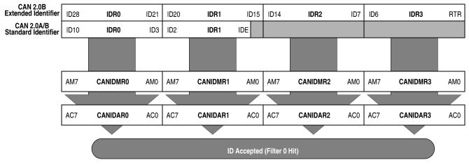
Figure 15-38. 32-bit Maskable Identifier Acceptance Filter
