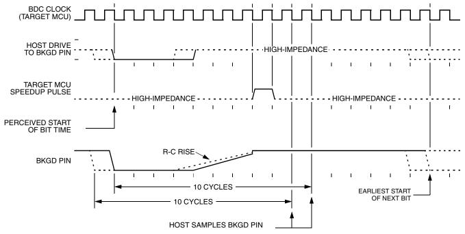
Figure 22-18. BDC Target-to-Host Serial Bit Timing (Logic 1)
