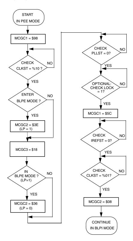
Figure 16-11. Flowchart of PEE to BLPI Mode Transition using an 8 MHz crystal
