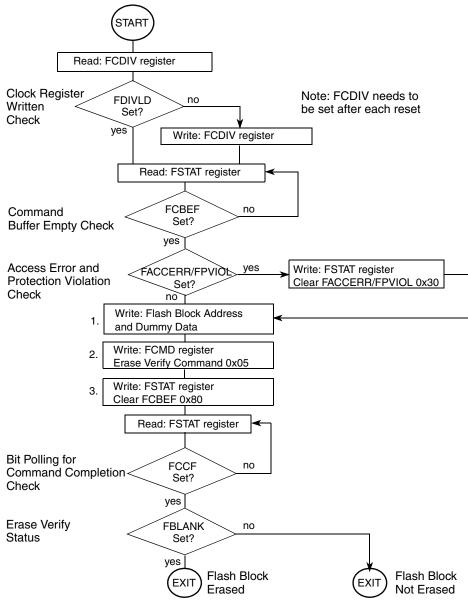
Figure 4-10. Example Erase Verify Command Flow
