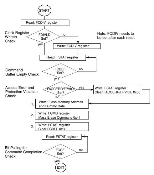
Figure 4-14. Example Mass Erase Command Flow
