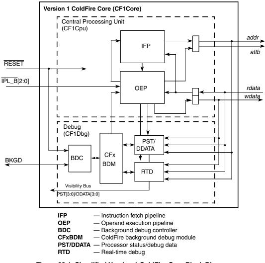
Figure 22-1. Simplified Version 1 ColdFire Core Block Diagram
