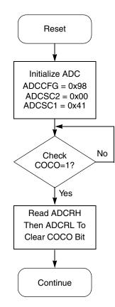
Figure 9-12. Initialization Flowchart for Example
