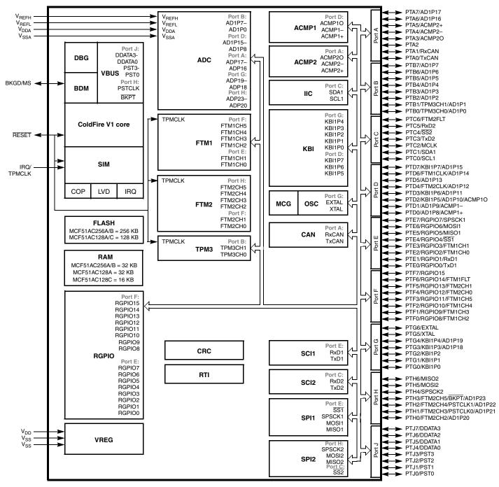
Figure 1-1. MCF51AC256 Series Block Diagram
