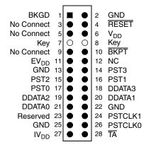
Figure 22-29. Recommended VBus BDM Connector
