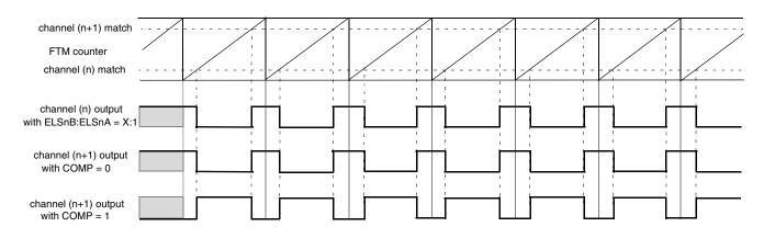
Figure 11-61. Channel (n+1) output in complementary mode with (ELSnB:ELSnA = X:1)
