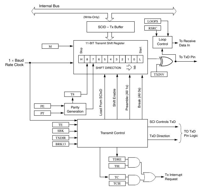
Figure 18-1. SCI Transmitter Block Diagram
