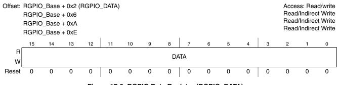
Figure 17-3. RGPIO Data Register (RGPIO\_DATA)
