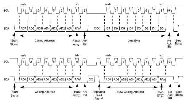
Figure 12-8. IIC Bus Transmission Signals
