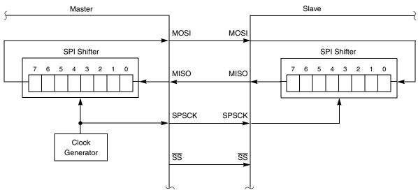
Figure 19-1. SPI System Connections
