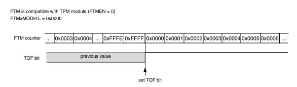
Figure 11-31. Example when the FTM counter is a free running
