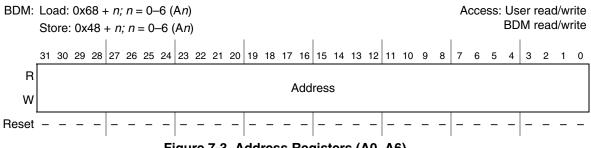
Figure 7-3. Address Registers (A0–A6)
