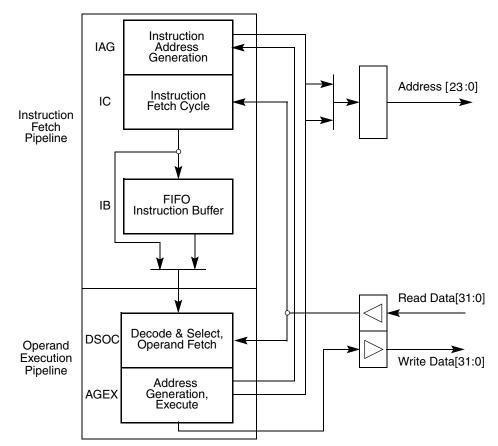
Figure 7-1. V1 ColdFire Core Pipelines
