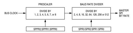
Figure 20-18. SPI Baud Rate Generation
