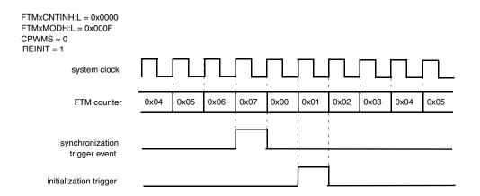
Figure 11-83. Initialization trigger generated when there is the synchronization trigger event and (REINIT = 1)
