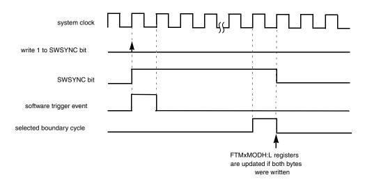
Figure 11-64. FTMxMODH:L synchronization when (REINIT = 0) and (software trigger was used)
