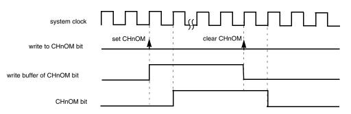
Figure 11-68. CHnOM synchronization when (SYNCHOM = 0)
