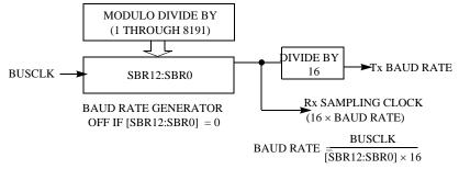
Figure 18-11. SCI Baud Rate Generation
