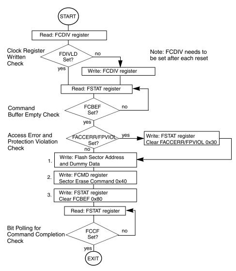
Figure 4-13. Example Sector Erase Command Flow
