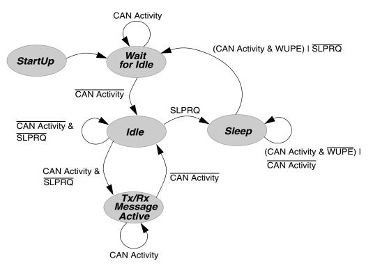
Figure 15-44. Simplified State Transitions for Entering/Leaving Sleep Mode
