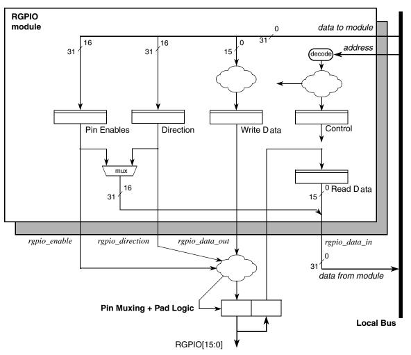
Figure 17-1. RGPIO Block Diagram
