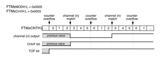
Figure 11-35. Example of the output compare mode when the match toggles the channel output
