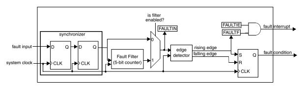
Figure 11-76. Fault Control Block Diagram
