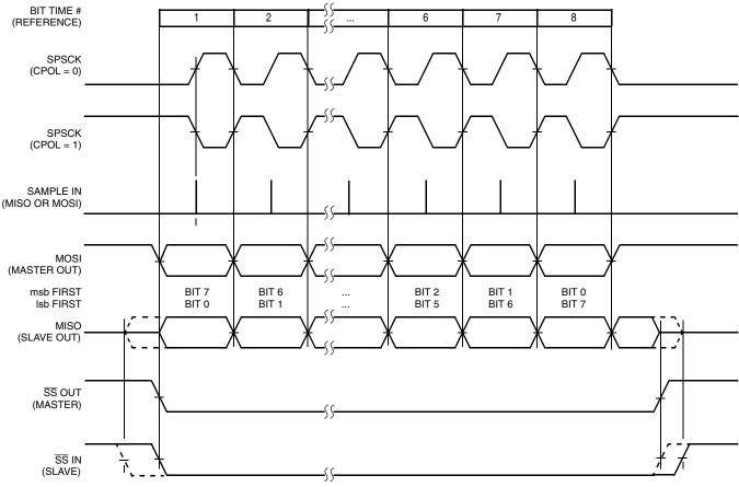
Figure 19-10. SPI Clock Formats (CPHA = 0)
