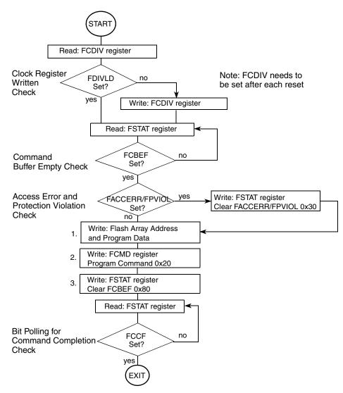
Figure 4-11. Example Program Command Flow
