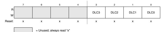
Figure 15-33. Data Length Register (DLR) — Extended Identifier Mapping
