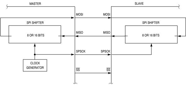
Figure 20-1. SPI System Connections
