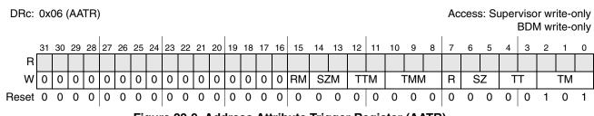
Figure 22-9. Address Attribute Trigger Register (AATR)
