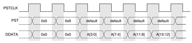
Figure 22-25. Example JMP Instruction Output on PST/DDATA
