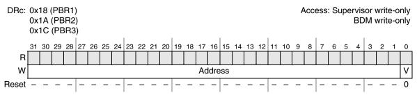
Figure 22-12. Program Counter Breakpoint Register n (PBRn, n = 1,2,3)
