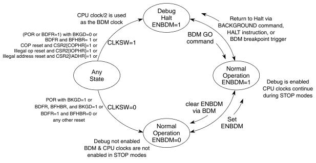
Figure 22-2. Debug Modes State Transition Diagram
