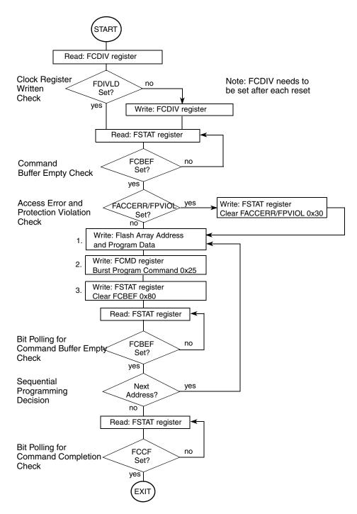
Figure 4-12. Example Burst Program Command Flow
