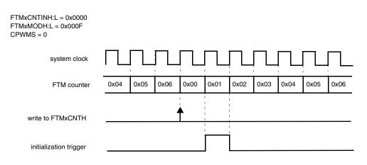
Figure 11-82. Initialization trigger generated when there is a write to FTMxCNTH (or FTMxCNTL)
