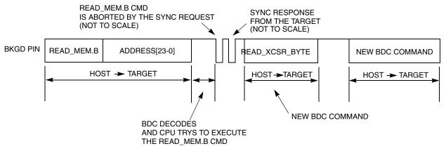
Figure 22-23. ACK Abort Procedure at the Command Level
