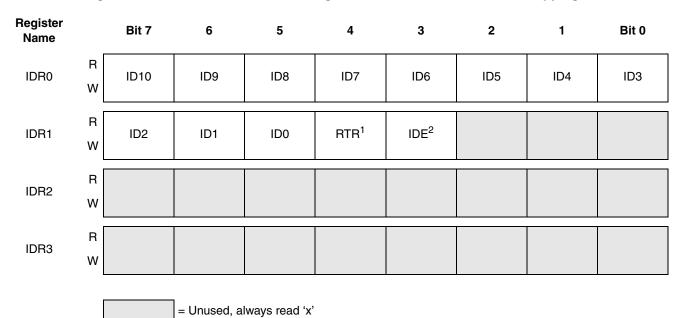
Figure 15-23. Receive/Transmit Message Buffer — Standard Identifier Mapping
