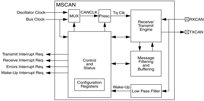
Figure 15-1. MSCAN Block Diagram
