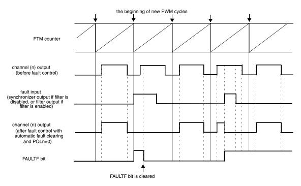
Figure 11-77. Fault control with automatic fault clearing
