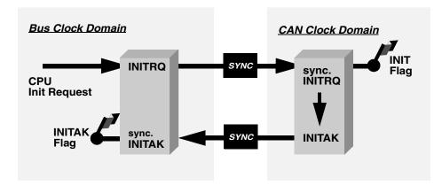
Figure 15-45. Initialization Request/Acknowledge Cycle
