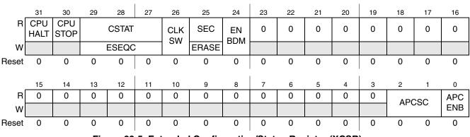
Figure 22-5. Extended Configuration/Status Register (XCSR)
