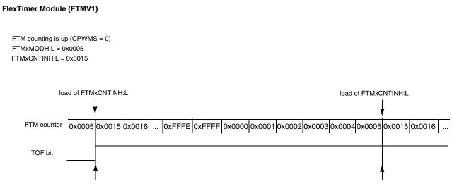
Figure 11-29. Example of up counting when the value of FTMxCNTINH:FTMxCNTINL registers is greater than the value of FTMxMODH:FTMxMODL registers
