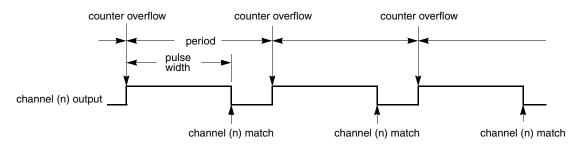
Figure 11-38. EPWM period and pulse width with ELSnB:ELSnA = 1:0
