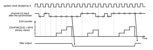
Figure 11-34. Channel input filter example
