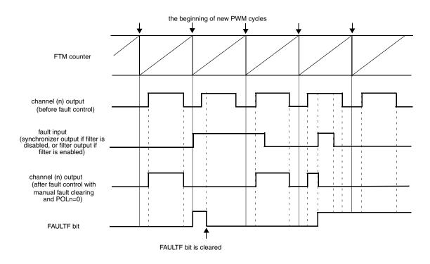
Figure 11-78. Fault control with manual fault clearing
