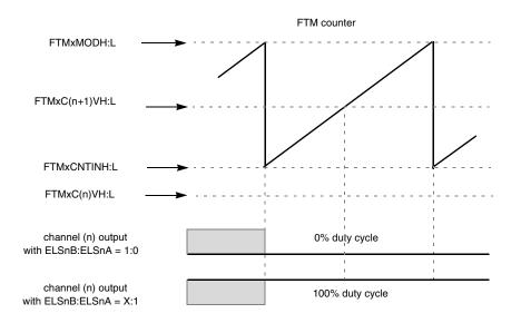
Figure 11-55. Channel (n) output if (FTMxC(n)VH:L < FTMxCNTINH:L) and (FTMxCNTINH:L < FTMxC(n+1)VH:L < FTMxMODH:L)
