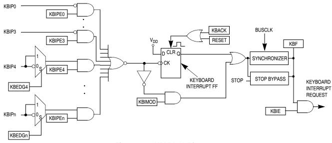
Figure 14-1. KBI Block Diagram
