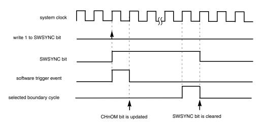
Figure 11-69. CHnOM synchronization when (SYNCHOM = 1) and (software trigger was used)
