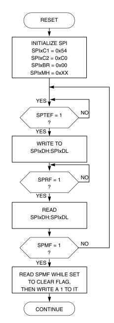
Figure 20-19. Initialization Flowchart Example for SPI Master Device in 16-Bit Mode for FIFOMODE = 0
