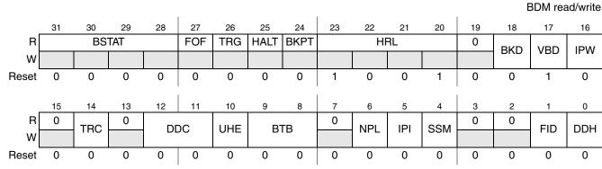
Figure 22-4. Configuration/Status Register (CSR)
