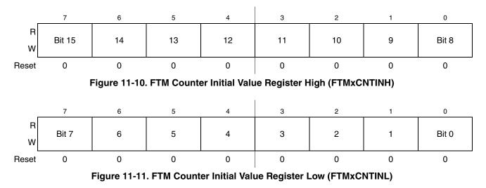
The first time that the FTM clock is selected (first write to change the CLKS[1:0] bits to a non-zero value), FTM counter will start with the value 0x0000. To avoid this behavior, before the first write to select the FTM clock, write the new value to the FTM counter initial value registers (FTMxCNTINH:FTMxCNTINL) and then initialize the FTM counter (write a value to FTMxCNTH or FTMxCNTL).
