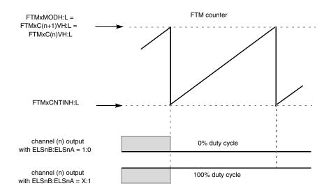
Figure 11-53. Channel (n) output if (FTMxC(n)VH:L = FTMxC(n+1)VH:L = FTMxMODH:L)
