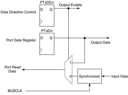
Figure 6-1. Classic Parallel I/O Block Diagram
