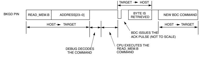
Figure 22-22. Handshake Protocol at Command Level
