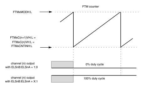
Figure 11-52. Channel (n) output if (FTMxC(n)VH:L = FTMxC(n+1)VH:L = FTMxCNTINH:L)
