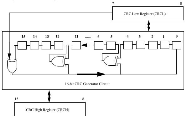
Figure 10-1. Cyclic Redundancy Check (CRC) Module Block Diagram
