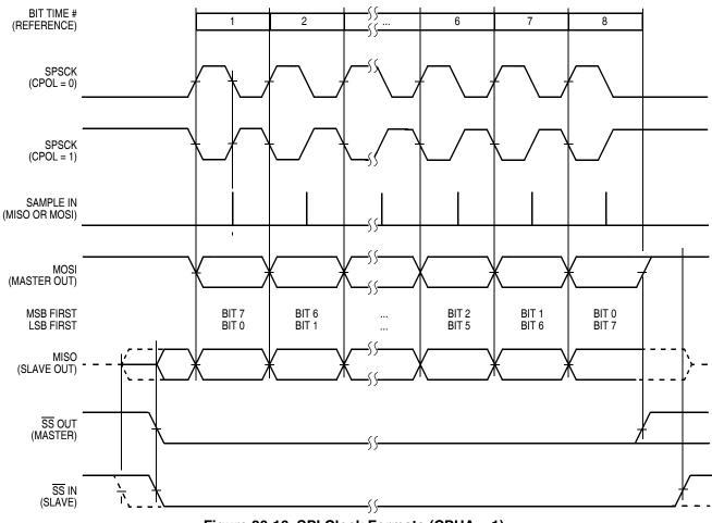
Figure 20-16. SPI Clock Formats (CPHA = 1)
