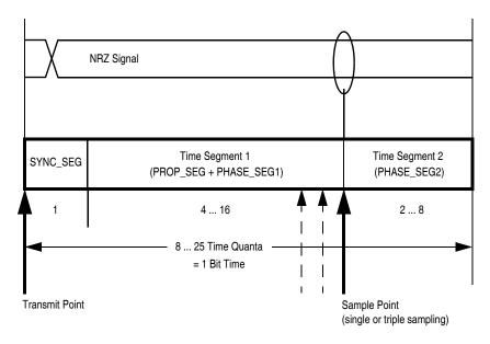
Figure 15-42. Segments within the Bit Time
