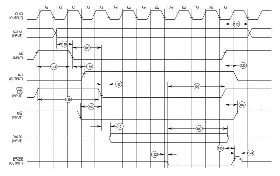
Figure 6-9. External Master Internal Asynchronous Write Cycle Timing Diagram
