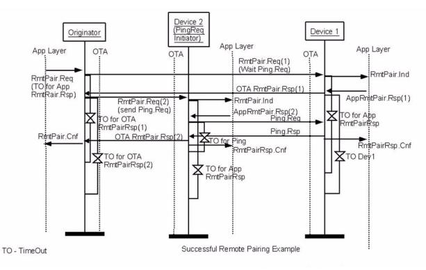
Figure 2-2. Successful Remote Pairing Example
