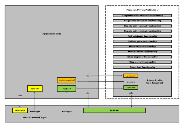
Figure 2-1. Private Profile Layer Components and Interfaces
