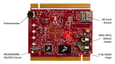
Figure 2: Back side of TWR-K70F120M module.
