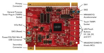
Figure 1: Front side of TWR-K60D100M module
