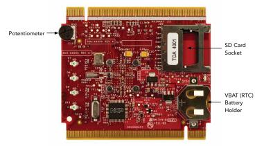
Figure 2: Back side of TWR-K60D100M module
