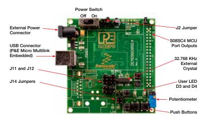
NOTE: For additional details, refer to the DEMO9S08SC4 User Manual and Board Schematics from the accompanying CD. You will find useful information such as default jumper settings and 9S08SC4 device signal mapping to the MCU port outputs.
