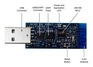
Figure 1: OM15080-JN5189 Board Components
