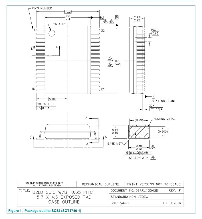
HSOP32, plastic, thermal enhanced small outline package; 32 terminals; 0.65 mm pitch; 7.5 mm x 11 mm x 2.22 mm body
