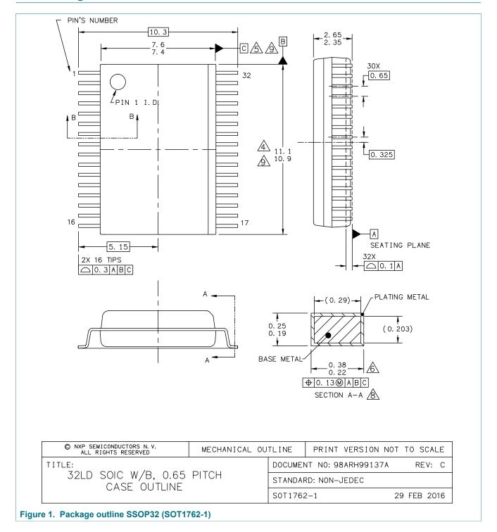
SSOP32, plastic, shrink small outline package; 32 terminals; 0.65 mm pitch; 7.5 mm x 11 mm x 2.5 mm
