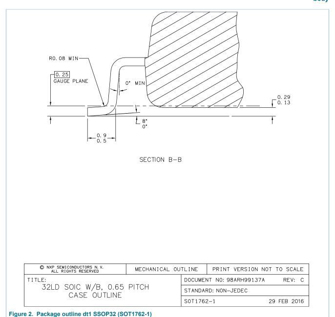
SSOP32, plastic, shrink small outline package; 32 terminals; 0.65 mm pitch; 7.5 mm x 11 mm x 2.5 mm body
