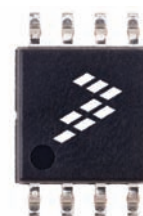
8-pin SOIC 3.9 mm x 4.9 mm body 50 mil/1.27 mm pitch
