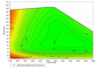
The NXP Inverter system was shown to produce a peak power of 220KW, and a max system efficiency of up to 96%.
