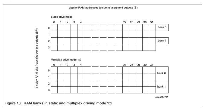
There are two banks; bank 0 and bank 1. <u>Figure 13</u> shows the location of these banks relative to the RAM map. Input and output banks can be set independently from one another with the Bank-select command (see <u>Table 9</u>). <u>Figure 14</u> shows the concept.
