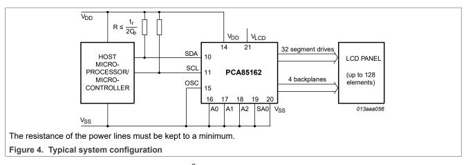
The host microcontroller maintains the 2-line  $I^2$ C-bus communication channel with the PCA85162. The internal oscillator is enabled by connecting pin OSC to pin V<sub>SS</sub>. The appropriate biasing voltages for the multiplexed LCD waveforms are generated internally. The only other connections required to complete the system are the power supplies (V<sub>DD</sub>, V<sub>SS</sub>, and V<sub>LCD</sub>) and the LCD panel chosen for the application.
