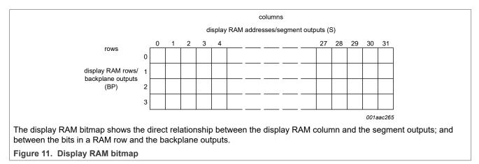
When display data is transmitted to the PCA85162, the display bytes received are stored in the display RAM in accordance with the selected LCD drive mode. The data is stored as it arrives and depending on the current multiplex drive mode the bits are stored singularly, in pairs, triples or quadruples. To illustrate the filling order, an example of a 7-segment numeric display showing all drive modes is given in Figure 12; the RAM filling organization depicted applies equally to other LCD types.
