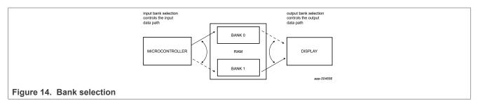
In the static drive mode, the bank-select command may request the contents of row 2 to be selected for display instead of the contents of row 0. In the 1:2 multiplex mode, the contents of rows 2 and 3 may be selected instead of rows 0 and 1. This gives the provision for preparing display information in an alternative bank and to be able to switch to it once it is assembled.
