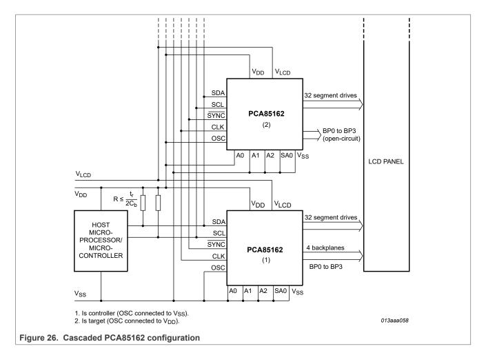
The <u>SYNC</u> line is provided to maintain the correct synchronization between all cascaded PCA85162. Synchronization is guaranteed after a power-on reset. The only time that <u>SYNC</u> is likely to be needed is if synchronization is accidentally lost (e.g. by noise in adverse electrical environments or by defining a multiplex drive mode when PCA85162 with different SA0 levels are cascaded).
