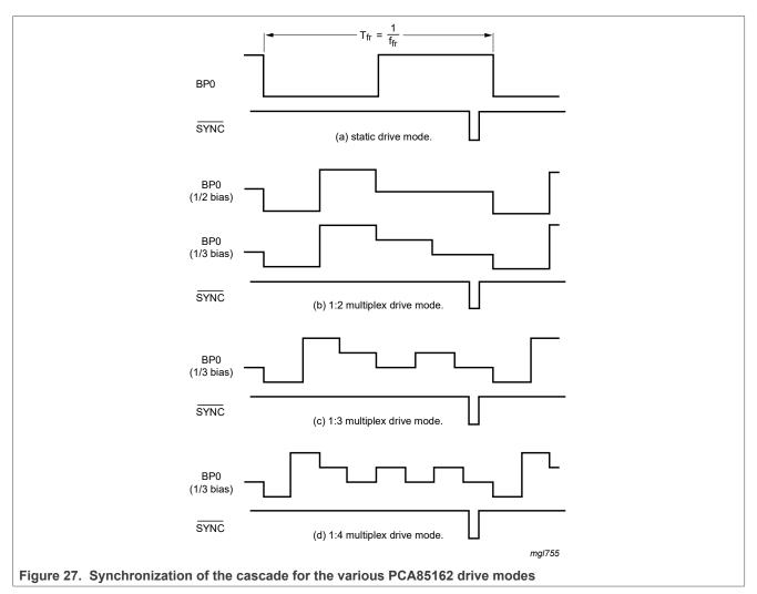
Only one controller, but multiple targets. are allowed in a cascade. All devices in the cascade have to use the same clock whether it is supplied externally or provided by the controller.
