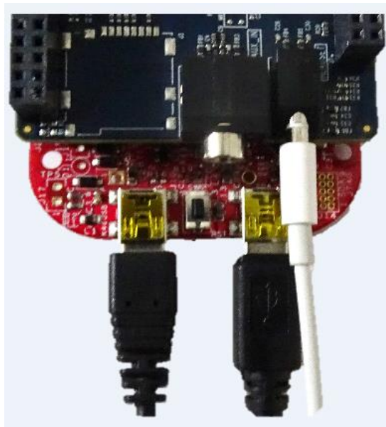
Figure 8. Speaker's connection to the audio codec shield
