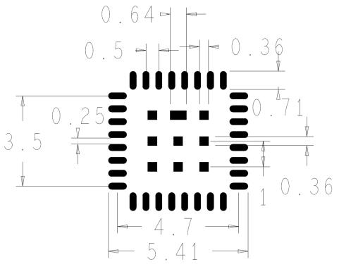
Figure 3. 41-pin MLGA solder stencil pattern
