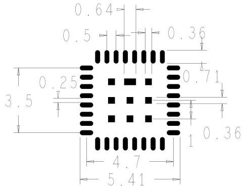
Figure 2. 41-pin MLGA solder mask pattern
