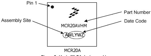
Figure 5. 41-pin MLGA device marking
