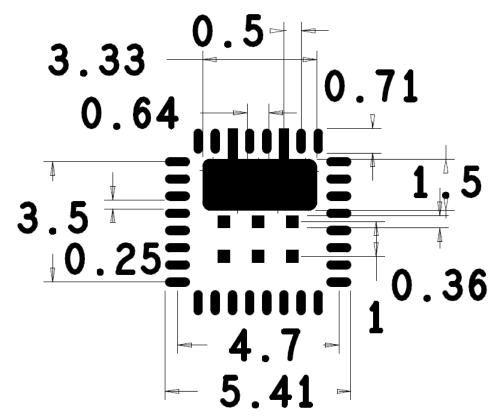
Figure 1. MLGA component copper layer
