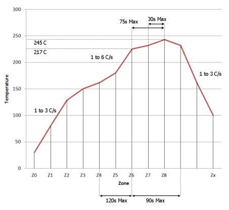
Figure 6. 41-pin MLGA soldering profile
