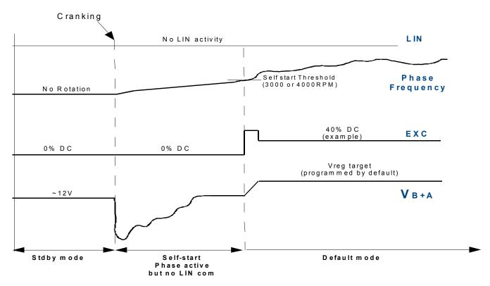
Figure 11. Self-start Operation (No LIN Communication)
