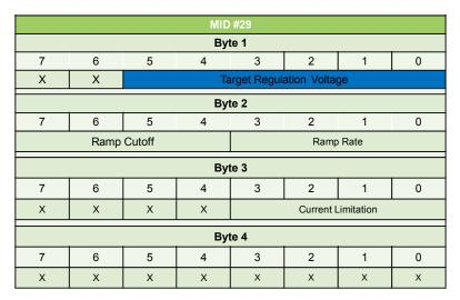
Figure 4. Target Regulation Voltage Data Location in MID#29
