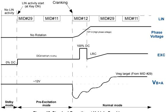
Figure 10. Standard Operation at Vehicle Cranking
