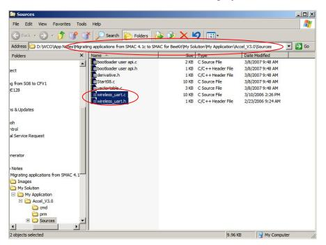
Figure 15. Paste Wireless UART files into the Accelerometer application folder
