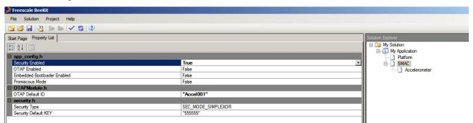
Figure 7 SMAC Software Component Configuration
