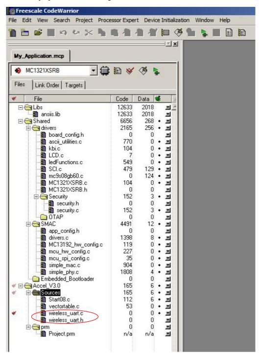
Figure 16. Adding the Wireless UART SMAC 4.1c files to the SMAC Codebase 1.0.4 Project
