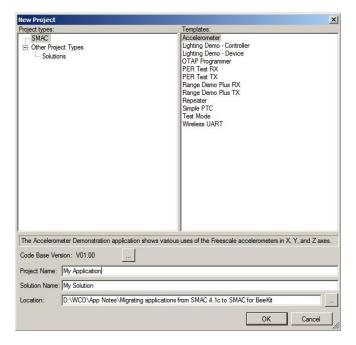
Figure 3. Naming an Accelerometer Project Template
