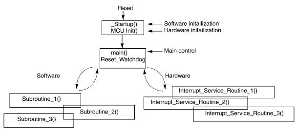
Figure 2. Blood Pressure Monitor Software Flow
