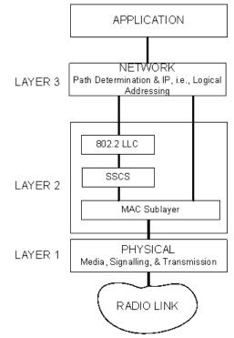
Figure A-2. The 7-Layer OSI Communication Model Adapted to the IEEE 802.15.4 Standard
