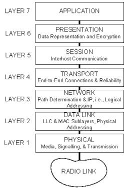
Figure A-1. The 7-Layer OSI Communication Model
