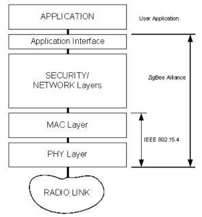
Figure A-3. The Communication Model Adapted to a ZigBee Stack
