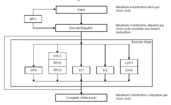
Figure 3. IBM 750CX/CXE Pipeline Diagram
