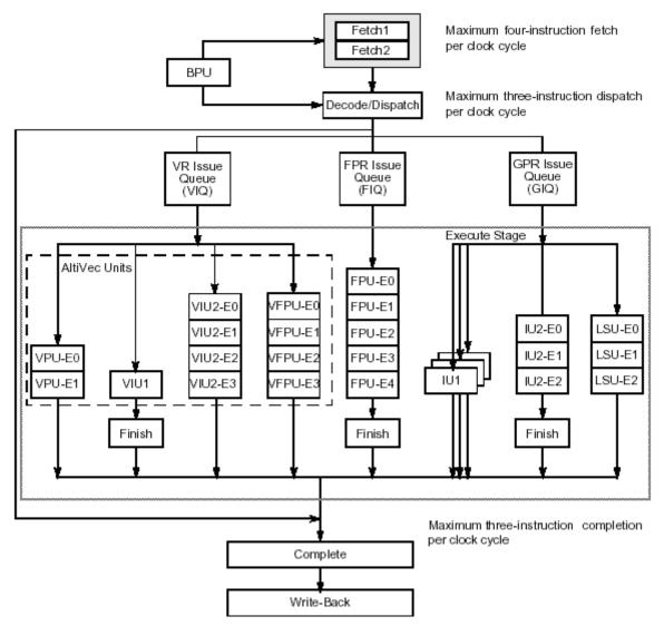
Figure 4. MPC7447A Pipeline Diagram
