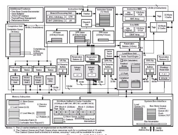
Figure 2. MPC7447A Core
