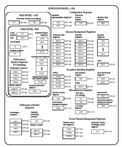
Figure 8. IBM 750CX/CXE Registers
