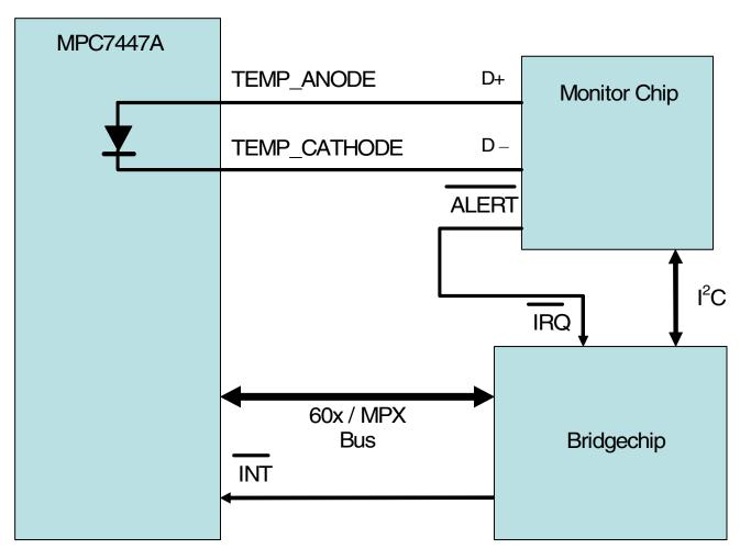
Figure 6. Temperature Monitoring Device Connection
