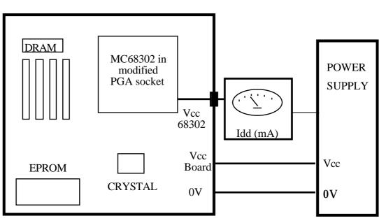
Figure 1. Power Test Set-Up
