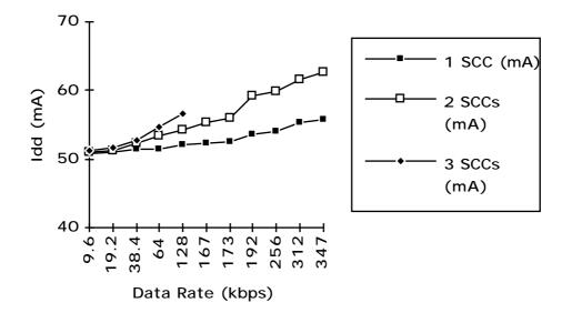
Graph 2b. UART Measurements for multiple SCCs at 16.67MHz.
