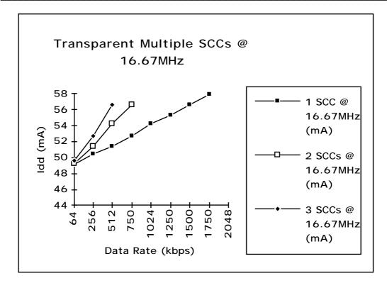
Graph 3b. Transparent Measurements for Multiple SCCs at 16.67MHz.
