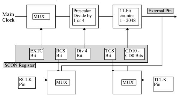
Figure 2. Baud Rate Generator.
