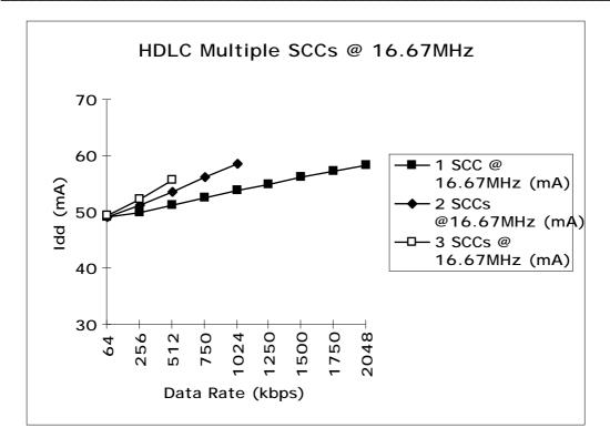
Graph 1b. HDLC Measurements for multiple SCCs at 16.67MHz.
