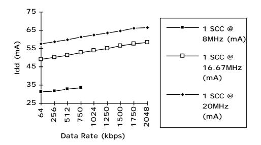
Graph 1a. HDLC Measurements for 1 SCC at 8, 16.67 and 20MHz.
