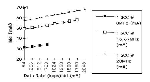
Graph 3a. Transparent Measurements for 1 SCC at 8, 16.67 and 20MHz.
