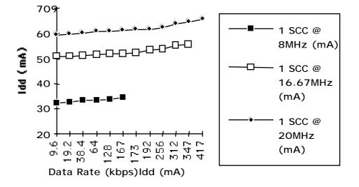
Graph 2a. UART Measurements for 1 SCC at 8, 16.67 and 20MHz.
