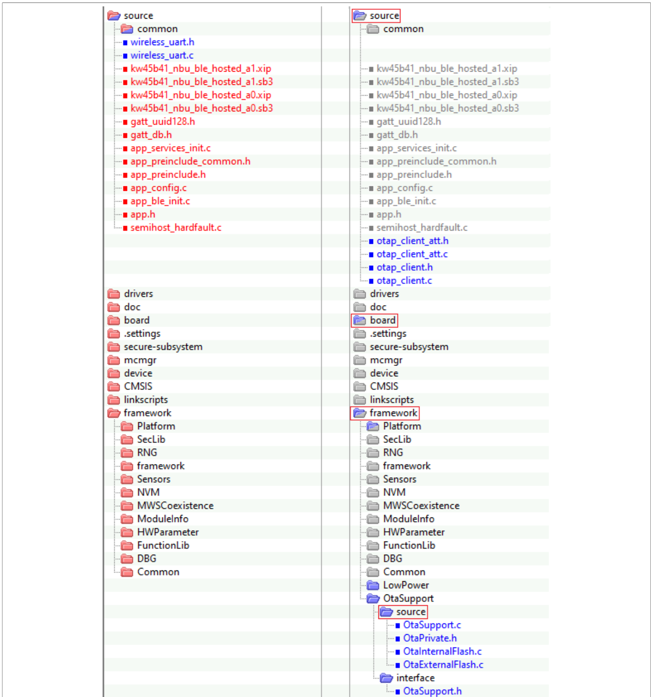
Figure 5. Files and folders highlighted in red are part of the OTAP client software, but not included in the Wireless UART
