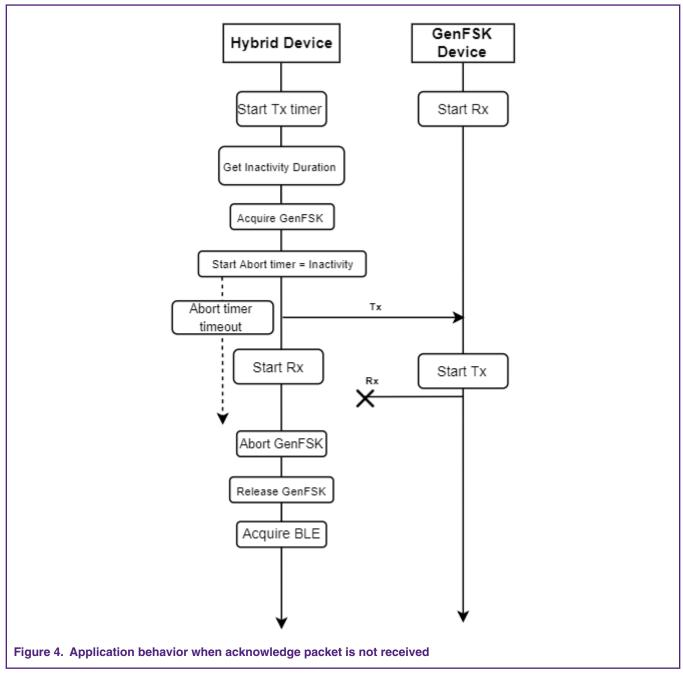
If the GenFSK Tx is successful but the Rx package has never been received during the abort timer, the abort Rx timer callback is triggered and it aborts any GenFSK activity to release the radio. Then, Bluetooth LE can acquire the radio.
