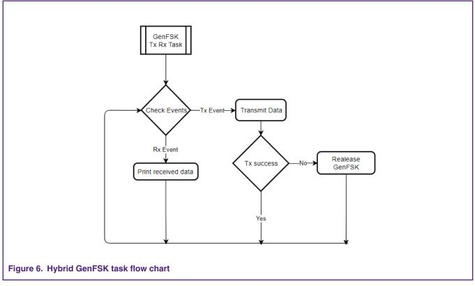
If a packet wasn't transmitted properly, GenFSK releases the radio and waits until the next TX timer interval to check the events to transmit a new packet.
