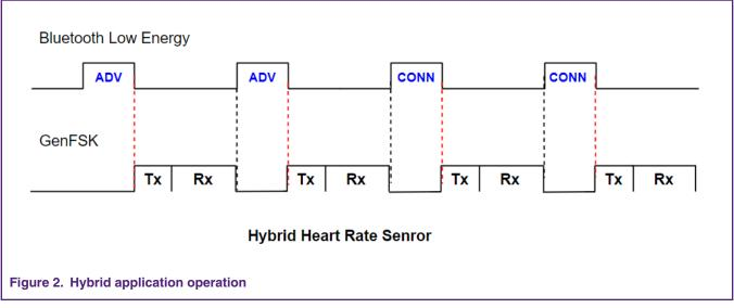
As shown in Figure 2 on page 4, the GenFSK operation is expected during the Bluetooth LE idle state. The GenFSK idle state is during advertising (ADV) or connection (CONN) events.
