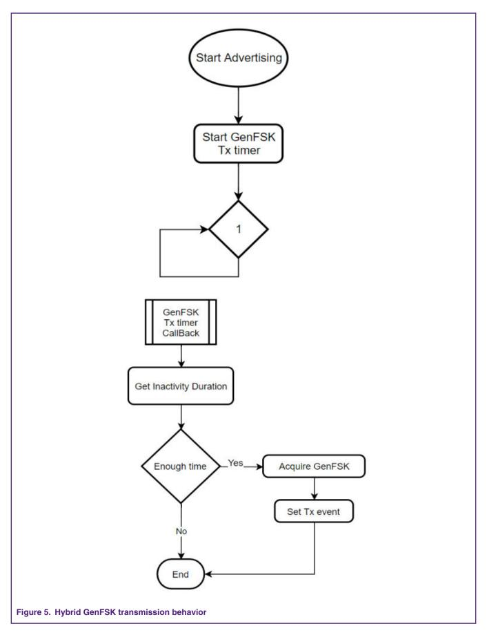
If GenFSK has enough time to execute, a Tx event is set, and a transmission packet is sent. The content of the packet depends on the Bluetooth LE status (connected, advertising or disconnected).
