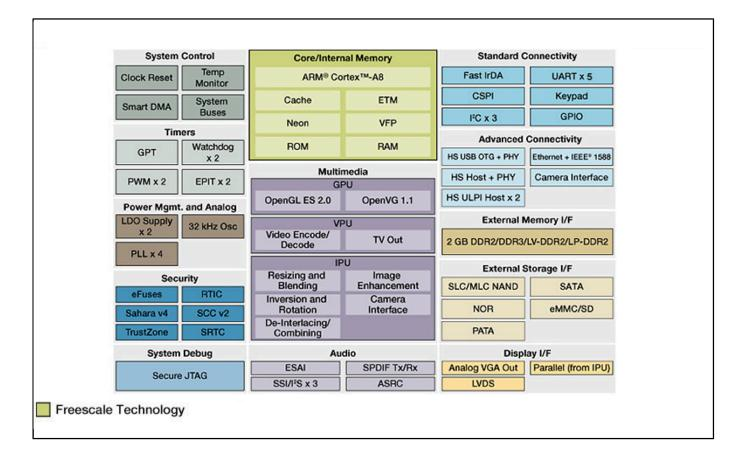
View additional information for Multimedia Applications Processors - HD Video, High-Performance, Low-Power, Arm® Cortex®-A8 Core.
