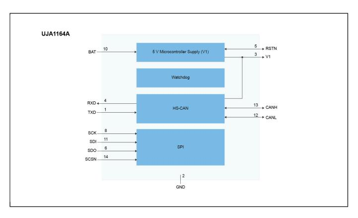
View additional information for Mini High-Speed CAN System Basis Chip with Standby Mode and Watchdog.
