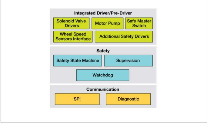
View additional information for Two-Wheel Antilock Braking (ABS) Controller for Motorcycles.
