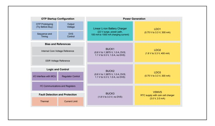
View additional information for PMIC with 1A Li+ Linear Battery Charger for Low Power Processor Systems.
