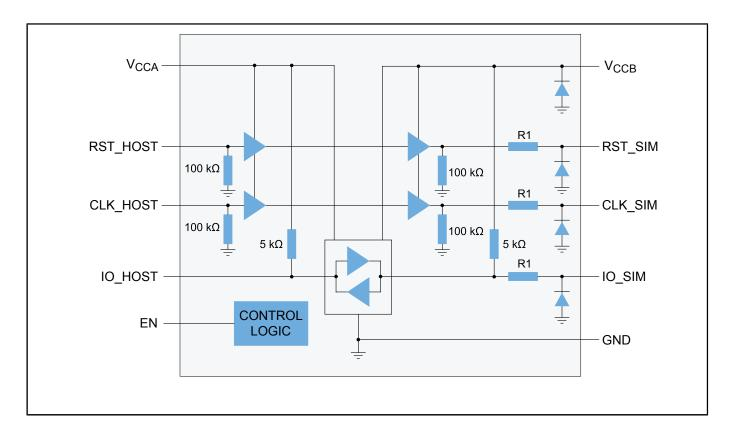
View additional information for SIM Card Interface Level Translator with EMI Filter and ESD Protection.
