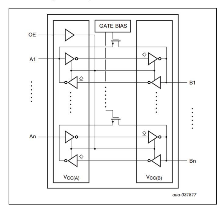
View additional information for 4-Bit Dual-Supply Translating Transceiver (Open-Drain, Auto-Direction Sensing).
