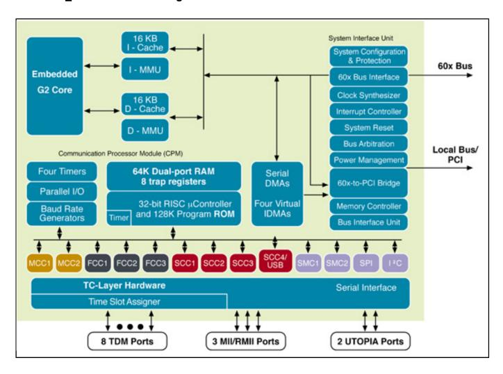
View additional information for PowerQUICC® II Processor with PCI, USB, 256-ch. HDLC, UTOPIA II Ports, 10/100 Ethernet, IMA.
